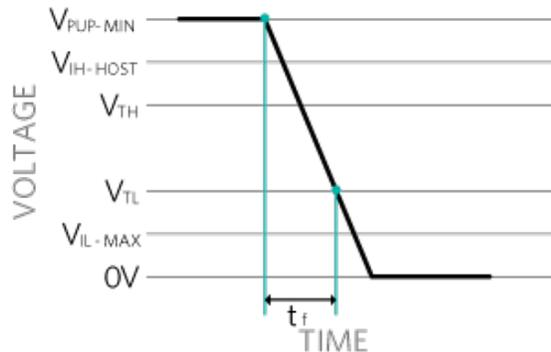
Figure 6. Time  $t_f$  to discharge total typical capacitance  $C_{TYP-TOTAL}$  from  $V_{PUP-MIN}$  to  $V_{TL}$ .
