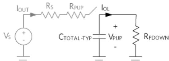
Figure 7. Simplified RC circuit that models the pull-down resistance  $R_{PDOWN}$  from either the 1-Wire host or device.  $I_{OL}$  is the pull-down current.
