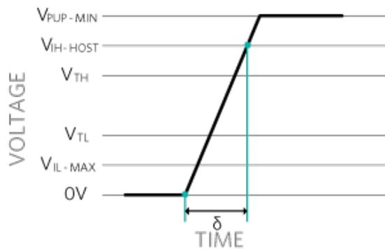
Figure 4. Time  $\delta$  to charge total typical capacitance  $C_{TYP-TOTAL}$  from 0V to  $V_{IH-HOST}$ .
