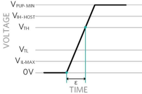
Figure 2. Time  $\epsilon$  to charge the total typical capacitance  $C_{TYP-TOTAL}$  from 0V to  $V_{TH}$ .
