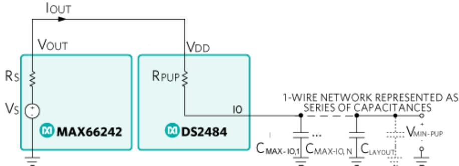
Figure 1. 1-Wire network modeled as a series of I/O capacitances  $C_{IO}$  and parasitic layout capacitance  $C_{LAYOUT}$  as a result of junctions on the 1-Wire node.
