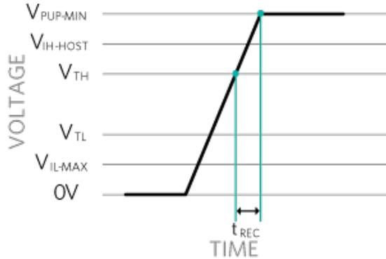
Figure 5. Shortest time  $t_{REC}$  possible to charge total typical capacitance  $C_{TYP-TOTAL}$  from  $V_{TH}$  to  $V_{PUP-MIN}$ .
