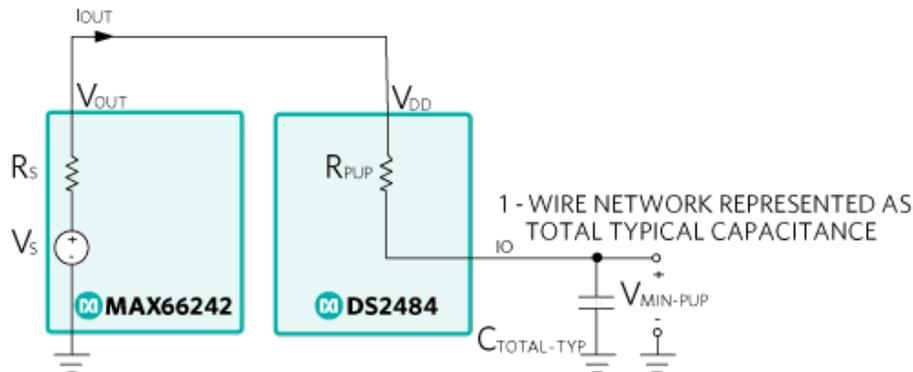
Figure 3. 1-Wire network modeled as an equivalent total typical capacitance  $C_{TOTAL-TYP}$  that includes the parasitic layout capacitance  $C_{LAYOUT}$ .
